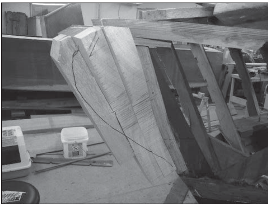
Triple lamination of 2" stock forms the bullnose.
