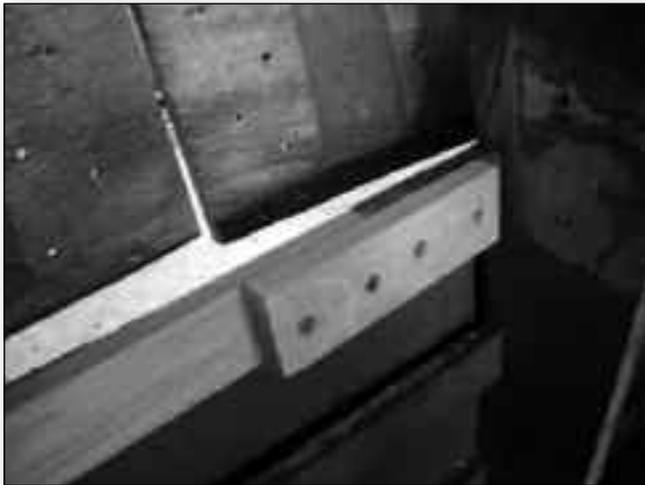
With the affected frame members replaced, it is time to remove the rotted edge on the planks and replace it with new wood. This will be an exercise in grain and wood color matching. Luckily, the line of the grain on the original plank had a slight upward angle to allow a long wedge to be removed in the rot area. A piece of wood was chosen with similar color and straight grain. A line was drawn with a straight
